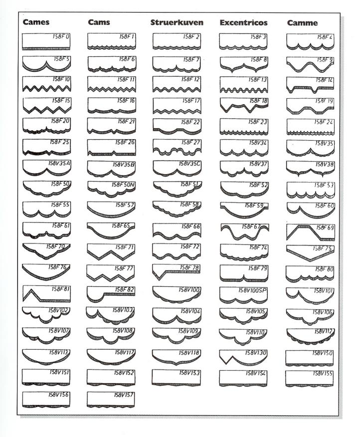
**Cams I 58 F:** needle spacing fixed during stitching. **Cams I 58 V:** needle spacing variable during stitching.
